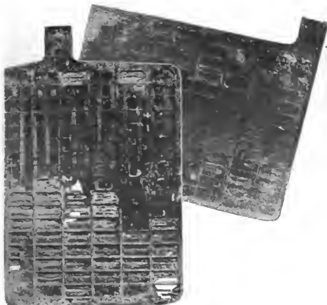
Fig. 12—Left—Frozen positive plate. The material is loosened and falls out, due to standing idle while discharged Fig. 13—Right—In a positive plate under the same circumstances the material becomes hard. Gray sulphate at top left corner is caused by broken-down insulation
